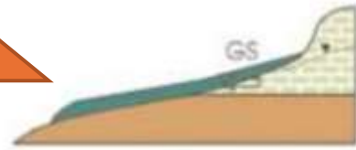
Groundwater seepage (Infiltration souterraine)
